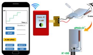
Figure 1. Schematic illustration of simultaneous detection on the ion-selective electrode (ISE) and Cl^- detection on the distance-based paper device (dPAD).
